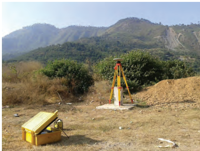
GPS Observation for providing Horizontal Control using Trimble GPS receiver at Rudraprayag, Uttarakhand.
