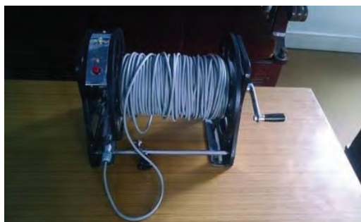
Low Cost Device measuring GW table
