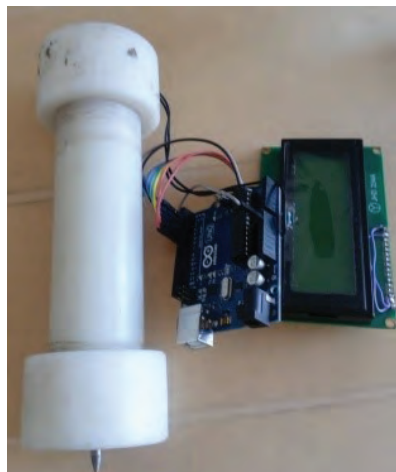
Prototype model of hand held fibre content measurement equipment
