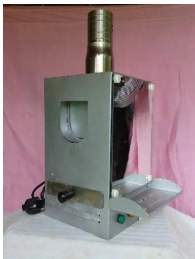
Incinerator for used Sanitary pads
