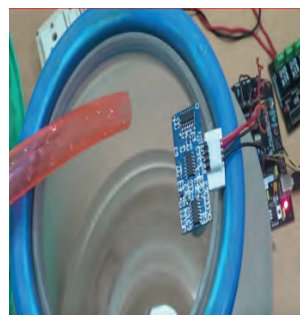
Embedded Water Level Measurement & Control System Experimental Setup
