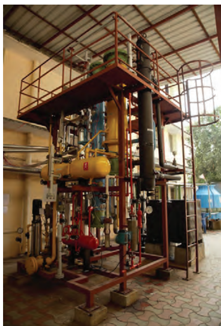
Combined power and cooling system that uses low-grade energy
