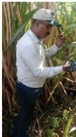
Operation of prototype model of hand held fibre content measurement equipment
