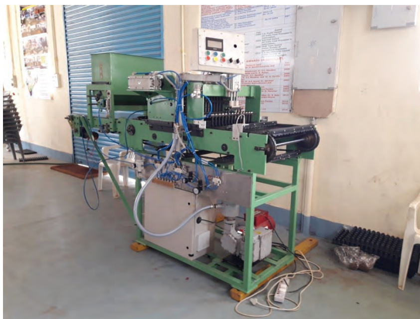
Automatic protray dibbling, sowing and topping machine
