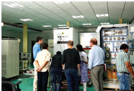
Fig.1: Factory Acceptance Test for Prototype Power Converters under progress
