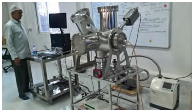
Fig. 2: Factory Acceptance Test of Ultra-High Vacuum Chambers in progress
